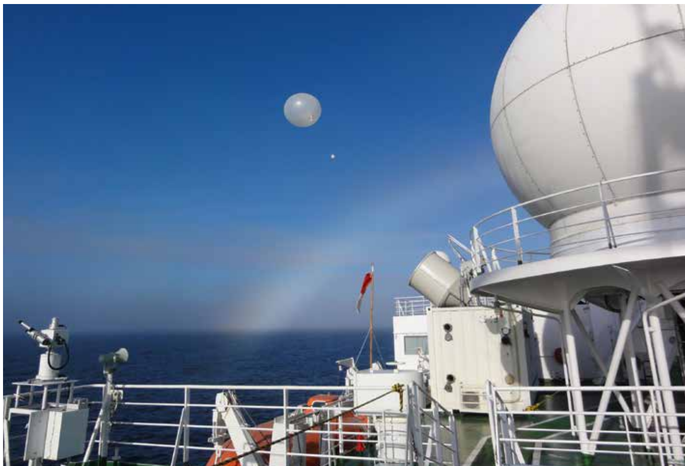
A radiosonde released into the air for aerological observation. Helium-filled balloons are used to lift radiosondes from more than 600 locations around the world twice a day. The small box-shaped device that functions as a weather station contains instruments for measuring atmospheric pressure, temperature, humidity, wind direction and speed and other parameters and transmits data by radio to a receiving station. "It is an old-fashioned observation tool. But, when used simultaneously at many locations, it helps you understand what is happening in the atmosphere," Inoue said. Photograph: Jun Inoue
